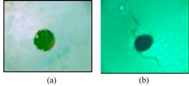
Figure 6 Holes observed in the elastomer membrane after puncture: (a) flat tip and (b) rounded tip.
