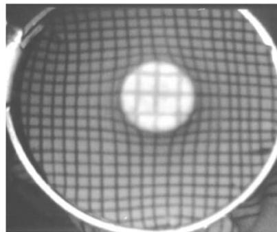
Figure 2 Deformations of the elastomer membrane for the cylindrical probes: (a) rounded tip and (b) flat tip.
