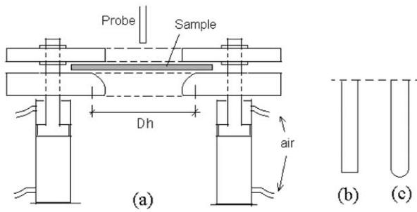
Figure 1 Sketch of sample holder (a); cylindrical probes with flat tip: (b); and cylindrical probes with rounded tip (c).
