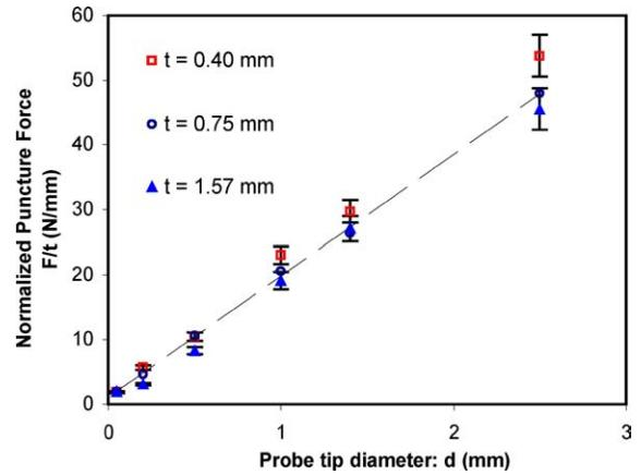
Figure 4 Normalized puncture force as a function of probe tip diameter for Neoprene sheets with different thicknesses.
