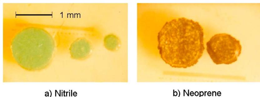
Figure 5 Cut-out disks of elastomer samples after puncture (optical microscopy: 20 $\times$ ).
